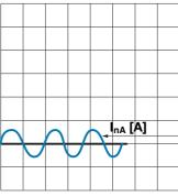
Compared with short-circuit currents, the rated current  $I_{nA}$  shown on the left is several times smaller.
