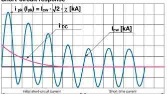
The rated peak withstand current  $I_{pk}$  and the rated short-time withstand current  $I_{cw}$  are the principal values for making a statement on the mechanical stability of a busbar system during an electrical short-circuit.
