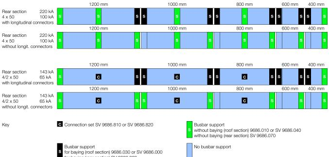
for baying (rear section) SV 9686.060 For sections up to 70 kA and width  $\leq$  800 mm and longitudinal
